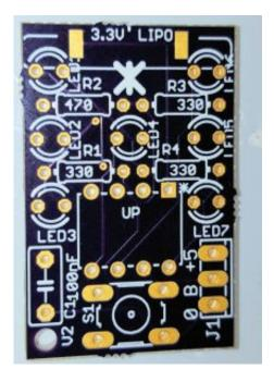
Take the PCB and ensure it is clean of fingerprints. This is the side the components go on.
