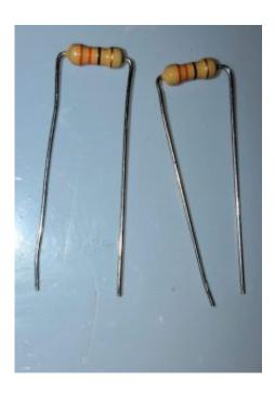
Find the 4 resistors and bend the legs as shown. There are three 330 ohm resistors (Orange Orange Brown) and one 470 ohm (Yellow Purple Brown)
