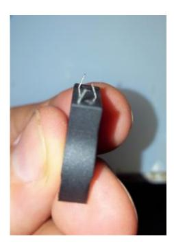
Find the battery holder and bend the legs of the holder as shown, It should fir over and under the PCB snugly with all three legs making contact with the pads on the PCB
