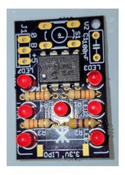
All of the LED's need to be placed with the cathodes (short leg) to the left hand side of the board in the picture on the left.
