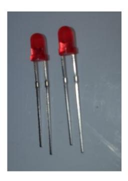
Find the 7 red LED's These must be placed in the PCB the correct way around. The short leg is the Cathode and the long leg is the cathode. If you have really good eyesight you will see the LED is a "D" shape with the flat side being cathode.
