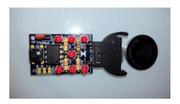
Place the battery into the holder making sure that +ve on the battery is uppermost (matching the + on the holder). Push the battery home.
