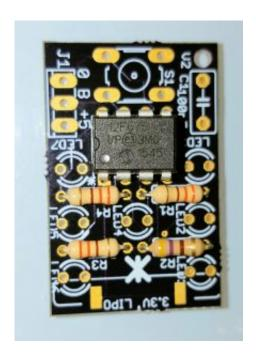
Place the 470 ohm (Yellow Purple Brown) in the resistor place holder labelled 470 (bottom right corner of this picture). Place the other 3 x 330 ohm (Orange Orange Brown) in the other resistor place holders labelled 330. When you are sure these are in the correct positions, solder them in place.
