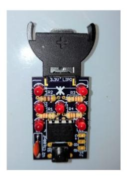
Check the position of the battery holder pins and solder to the three pads (two on top, one below)
