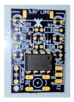
Put in the IC (black 8 legs) the little circular dot needs to be positioned nearest the square pad (top right of the IC with the board this way up). Check this orientation again, and if you are happy, solder in the IC, beign careful not to bridge any connections.
