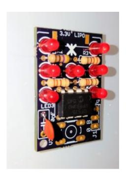
When you have placed and soldered all of the LED's add in the 100nF capacitor.
